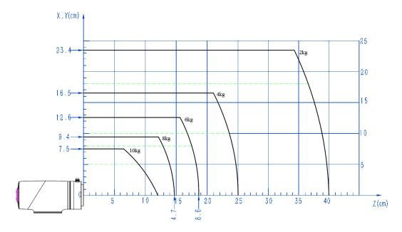
Figure 5.16 CR10 load curve
