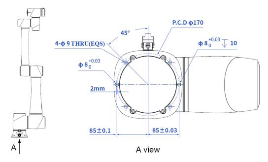
Figure 5.14 CR10 base installation dimensions
