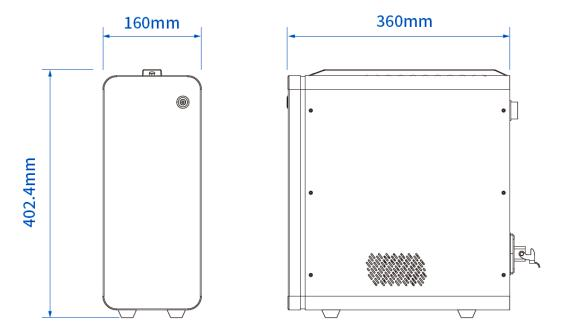
Figure 5.25 Controller dimensions
