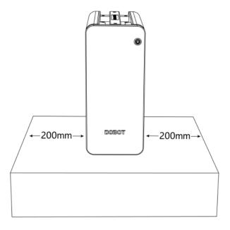
Figure 7.3 Controller installation space requirement
