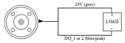
Figure 6.20 End DO wiring
