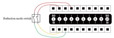
Figure 6.15 SI connected to reduction mode switch
