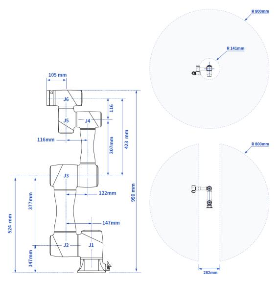
Figure 5.9 CR7 dimensions and working space
