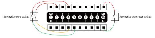
Figure 6.14 SI connected to protective stop device (with reset switch)
