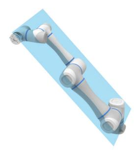
Figure 4.6 Elbow singularity
