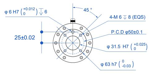
Figure 5.11 End flange dimensions
