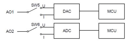
Figure C.4 Analog output simple circuit
