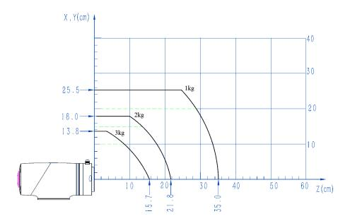
Figure 5.4 CR3 load curve
