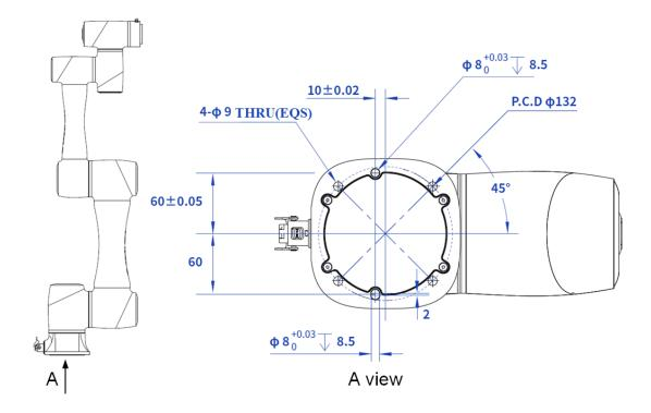
Figure 5.10 CR7 base installation dimensions
