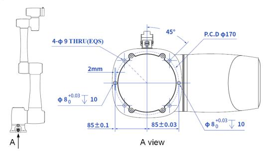
Figure 5.18 CR12 base installation dimensions
