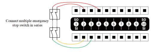
Figure 6.13 SI connected to multiple emergency stop switches
