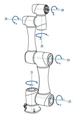
Figure 4.1 Joint coordinate system
