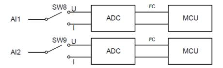
Figure C.3 Analog input simple circuit
