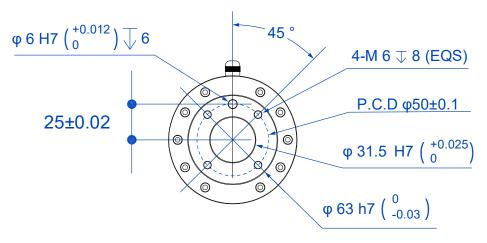
Figure 5.3 End flange dimensions
