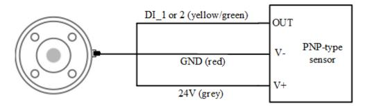
Figure 6.19 End DI wiring (3-wire senosr)
