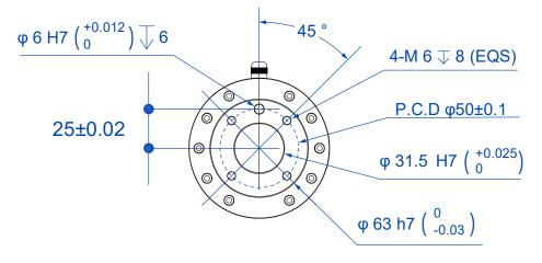
Figure 5.7 End flange dimensions
