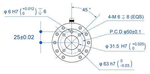
Figure 5.15 End flange dimensions
