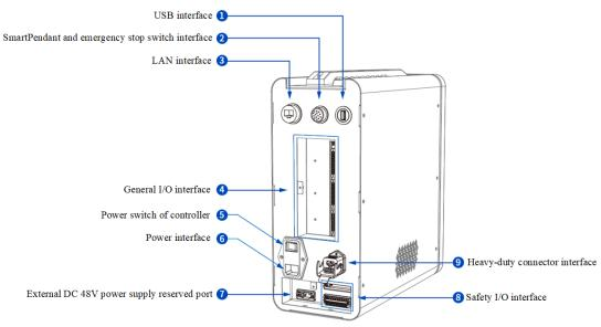
Figure 6.1 Controller electrical interfaces
