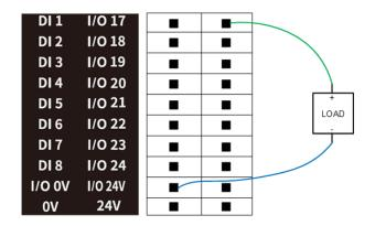
Figure 6.7 DO connected to external load
