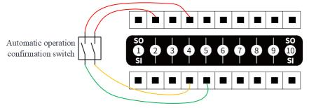
Figure 6.16 SI connected to automatic operation confirmation switch
