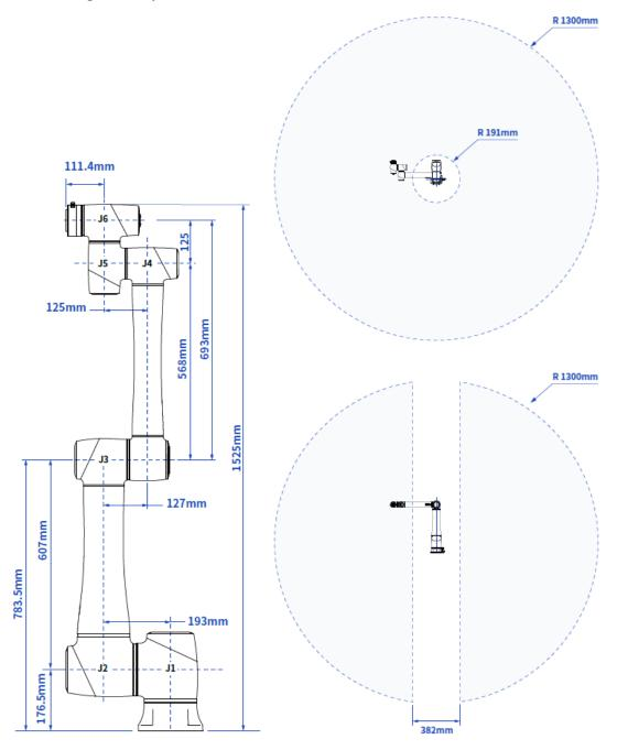
Figure 5.13 CR10 dimensions and working space
