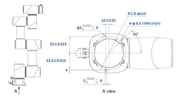
Figure 5.2 CR3 base installation dimensions
