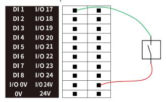
Figure 6.5 DI connected to PNP-type input
