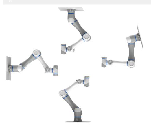
Figure 7.1 CR robot installation posture
