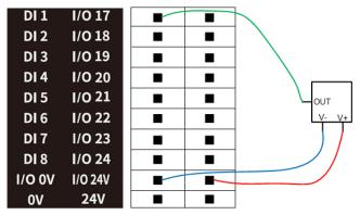
Figure 6.6 DI connected to PNP-type input
