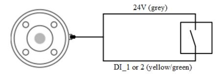
Figure 6.18 End DI wiring (simple switch)
