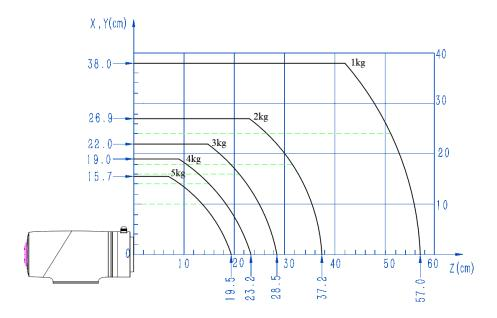
Figure 5.8 CR5 load curve
