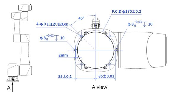
Figure 5.22 CR16 base installation dimensions
