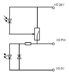
Figure C.2 Multiplexed digital input/output simple circuit
