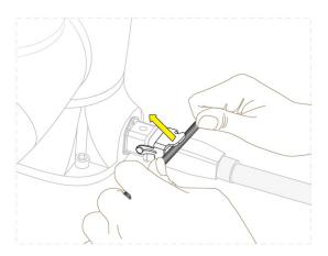
Figure 7.6 Unlock the heavy-duty connector
