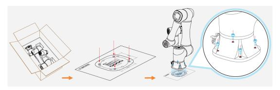
Figure 7.2 Base installation
