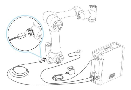
Figure 7.4 Wiring diagram
