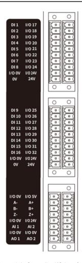
Figure 6.2 Controller I/O interface
