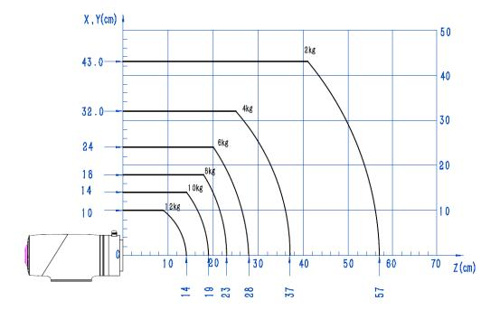
Figure 5.20 CR12 load curve
