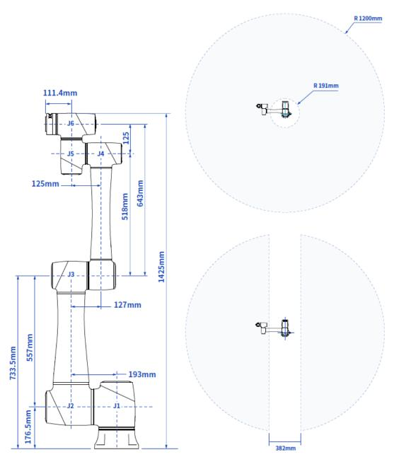
Figure 5.17 CR12 dimensions and working space
