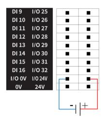
Figure 6.4 I/O connected to external power supply
