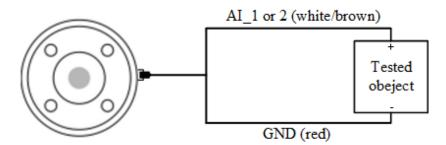
Figure 6.21 End AI wiring
