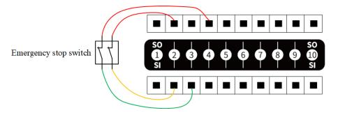
Figure 6.12 SI connected to an emergency stop switch
