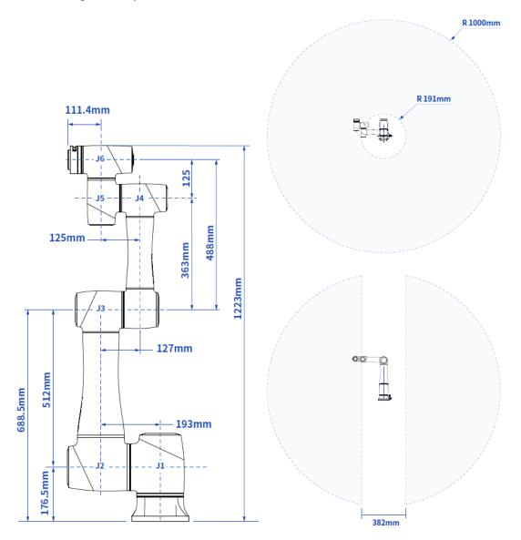
Figure 5.21 CR16 dimensions and working space
