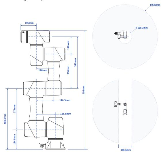
Figure 5.1 CR3 dimensions and working space
