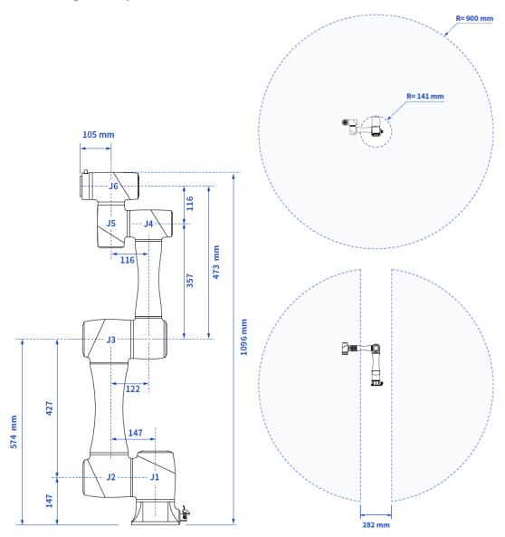
Figure 5.5 CR5 dimensions and working space
