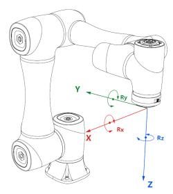
Figure 4.3 Tool coordinate system
