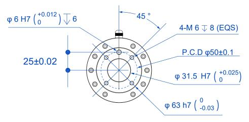
Figure 5.23 End flange dimensions
