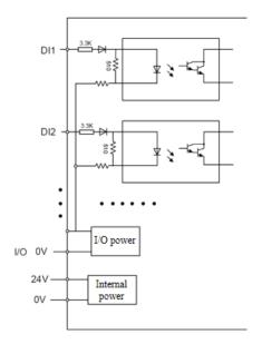
Figure C.1 Digital input simple internal circuit
