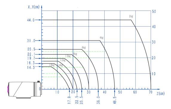
Figure 5.24 CR16 load curve
