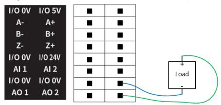
Figure 6.11 AO connected to external load
