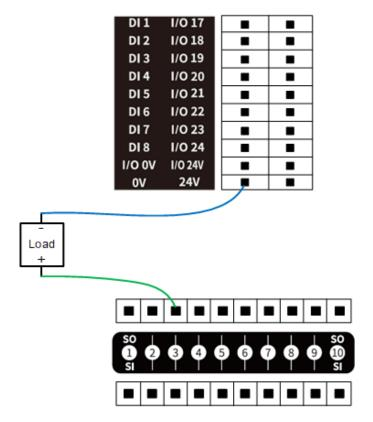
Figure 6.17 SO connected to external load
