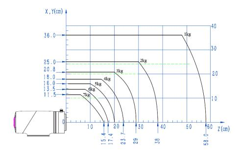
Figure 5.12 CR7 load curve
