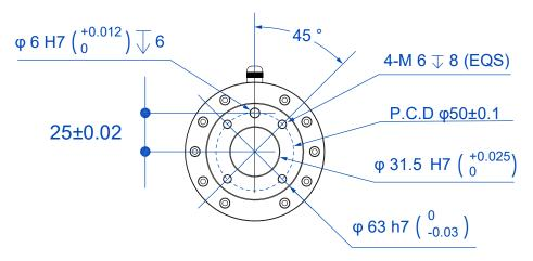
Figure 5.19 End flange dimensions
