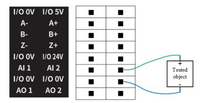
Figure 6.9 Al connected to tested object
