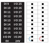
Figure 6.3 I/O using internal power supply
